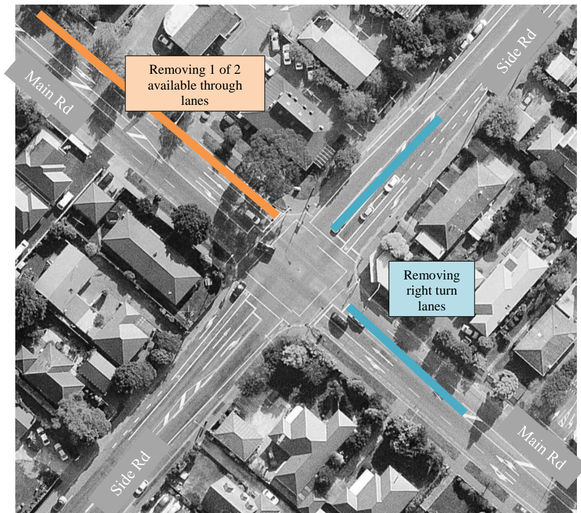
Figure 10: Typical 4-Way Moderate Signals
