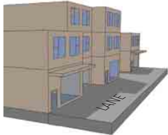
Broken facade weakens lane edge
