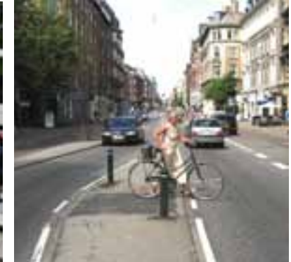
Two way streets with a refuges give better crossing possibilities. The waiting area improves safety and comfort for pedestrians. Gammel Kongevej, Copenhagen
