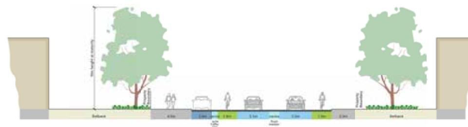
Figure 68 - Indicative road cross-section at Ferrymead illustrating the impact that larger-scale tree planting would have on this section of the corridor. Planting would be subject to agreements with private property owners.
