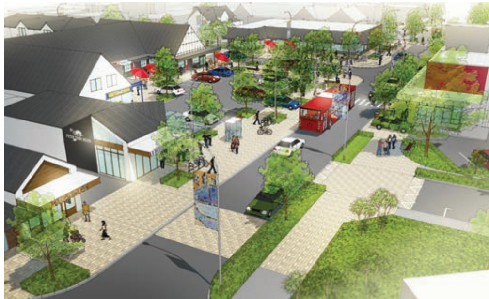
Figure 6b – View along Edgeware Road looking west, showing widened footpath and shorter crossing distances for pedestrians.
