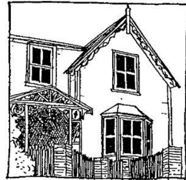
Drawing 51: Weatherboard house with decorative timber trim
