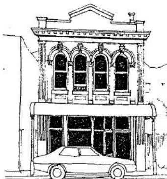
Drawing 50: Painted masonry façade with decorative plaster cornices and trim
