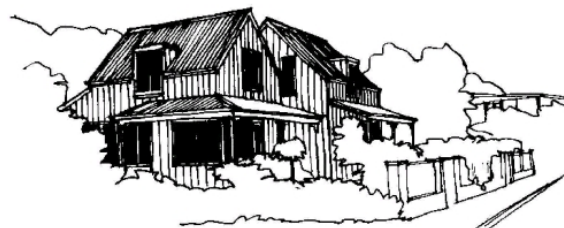
Multiple Gable Ends Roofs
