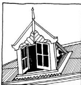
Dormer in a roof
