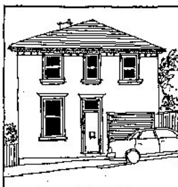
2 storey hip roof
