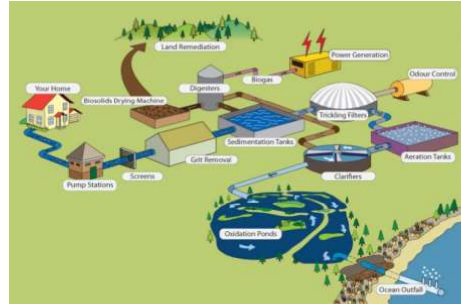
Wastewater Treatment Process
