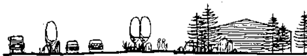
Separation of on-site vehicles and pedestrian movement is desirable for safety and amenity.
