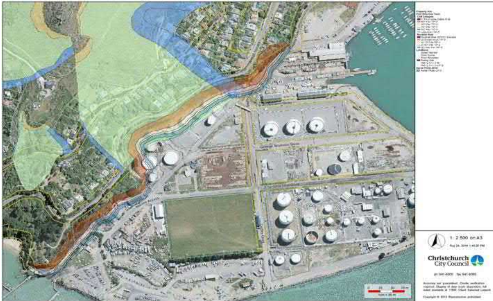
Figure F. 7: Combined map showing AIFR from Cliff Collapse and Rockfall (supplied by CCC)
