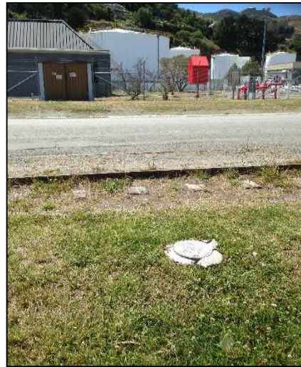
Photo 11: Groundwater monitoring well
