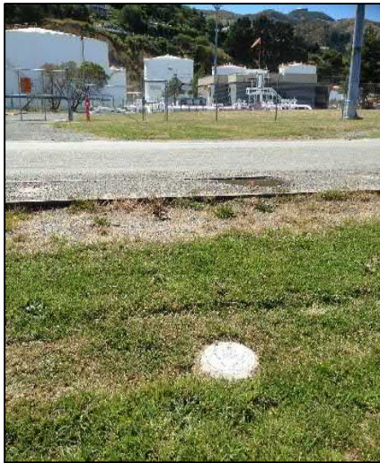
Photo 10: Groundwater monitoring well
