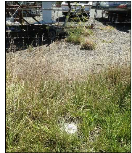
Photo 12: Groundwater monitoring well
