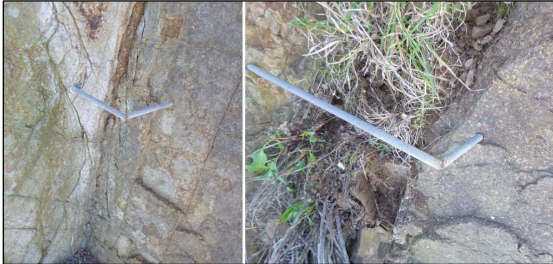
Figure 3 Current condition of two of the monitoring bolts installed at Naval Point in 2012
