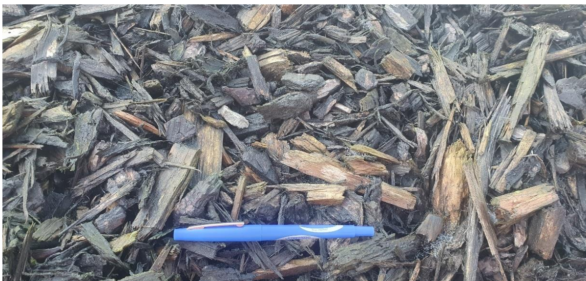
Figure 2.4: Biofilter media after replacement (right) in 2023.
