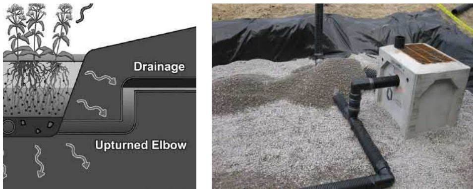
Figure 19 Submerged Zone schematic and installation photo (Brown et al, 2009)
