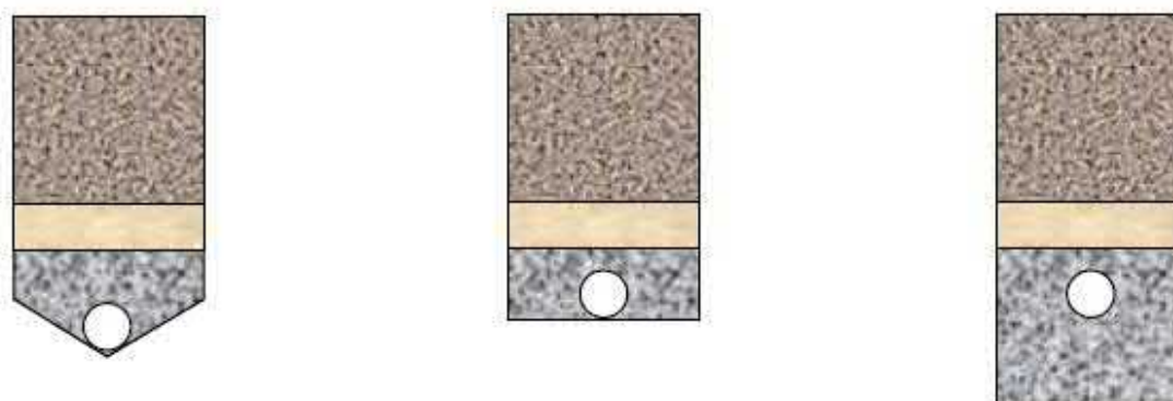
Figure 16 Drainage Layer Base Profile
