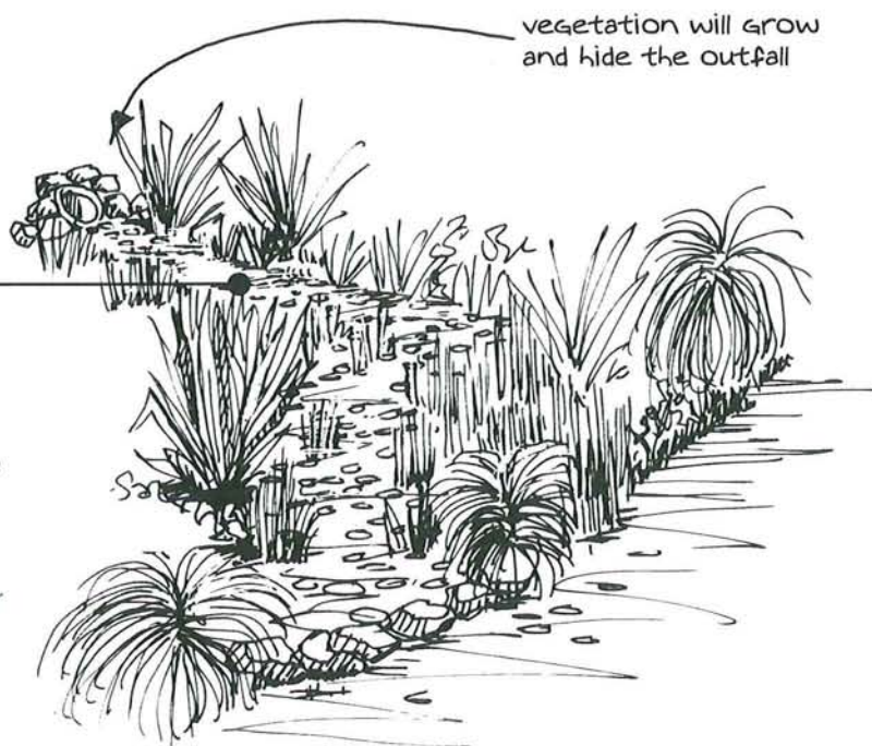
Figure 9-17: Stormwater outfalls can be set back from the waterway bank and planted. When the vegetation grows, the outfall pipe will be hidden from view, and the vegetation will help to trap litter and some sediment prior to stormwater entering the stream. This sketch illustrates a possible design for a low stormwater outfall.
