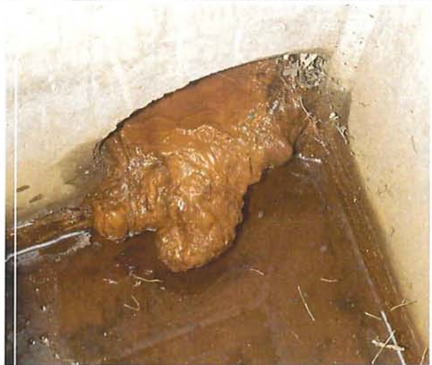
Figure 5-4A: The iron reducing bacterium Thiobacillus ferro-oxidaans can form filamentous threads.
