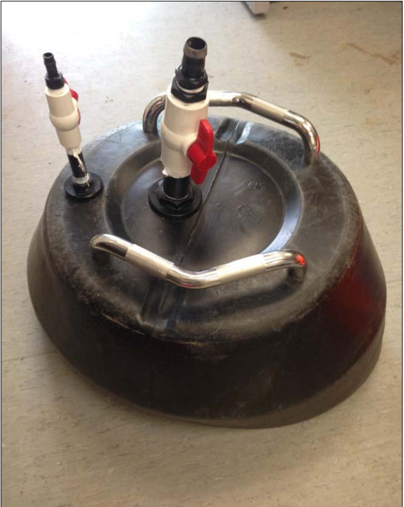
Figure 12a: Large Spring Vent Seepage Meter
