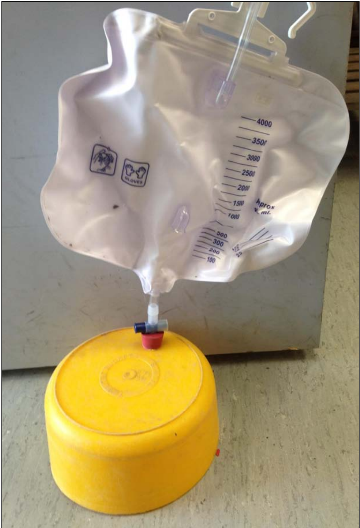
Figure 12b: General Streambed Seepage Meter
