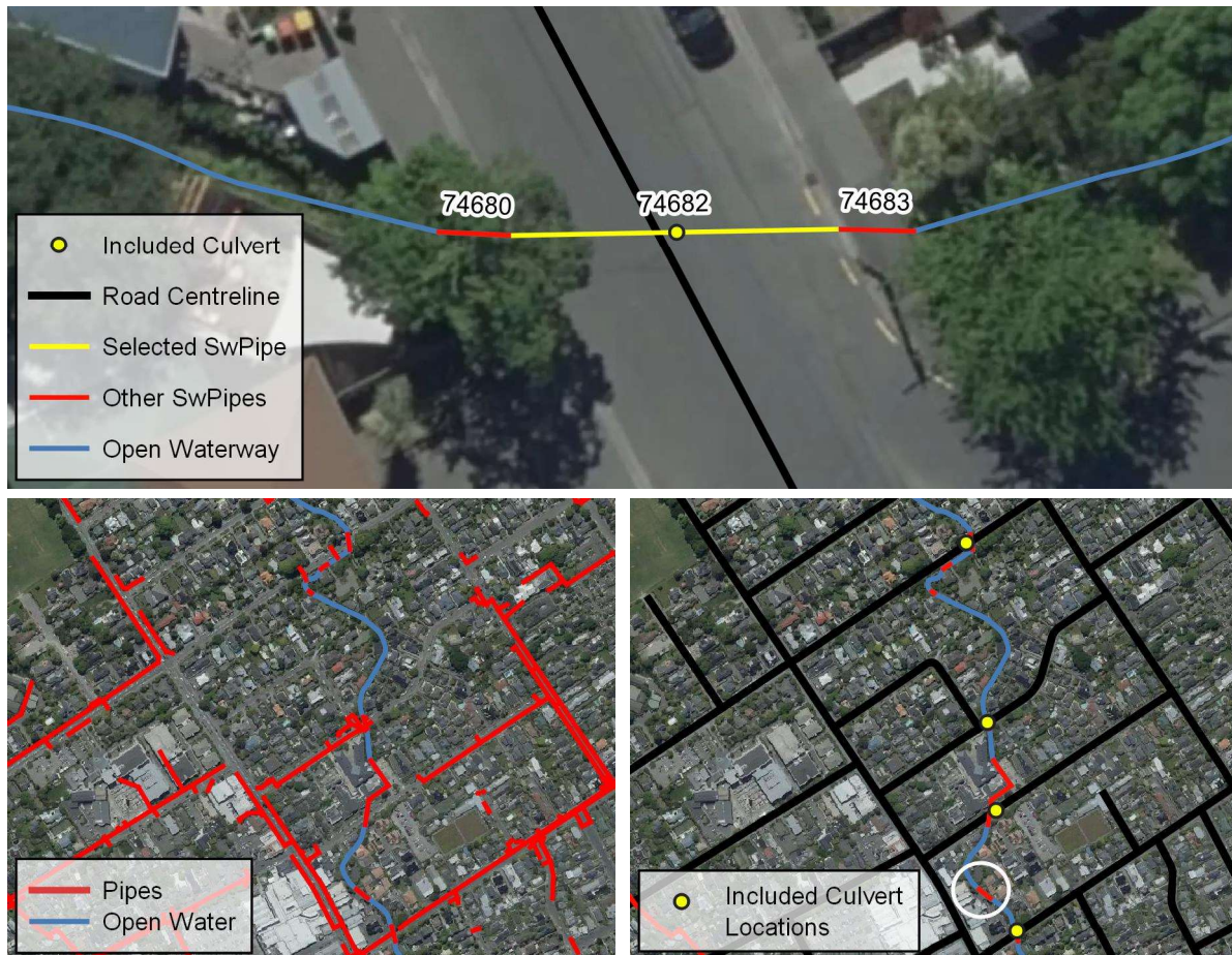
Figure 1: The selection of a single culvert asset by intersecting the layer with road centrelines, for which points were created (top). Pipes that were not on CCC watercourse lines (bottom left) were excluded (bottom right), reducing noise in the dataset. Note that this method does not capture pipes that do not intersect roads, as highlighted by the white circle on the bottom right map.
