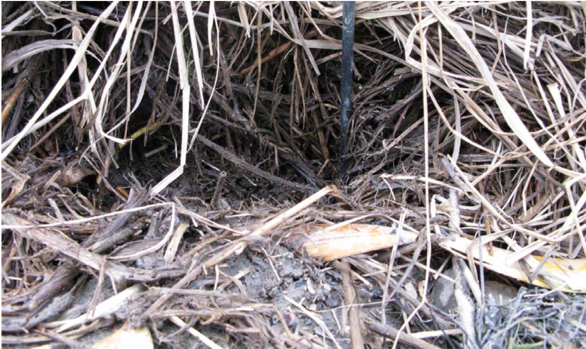
Figure 15. At this location, the original soil level, and grass root hair matrix, has been buried under about 10 cm of liquefaction silt.
