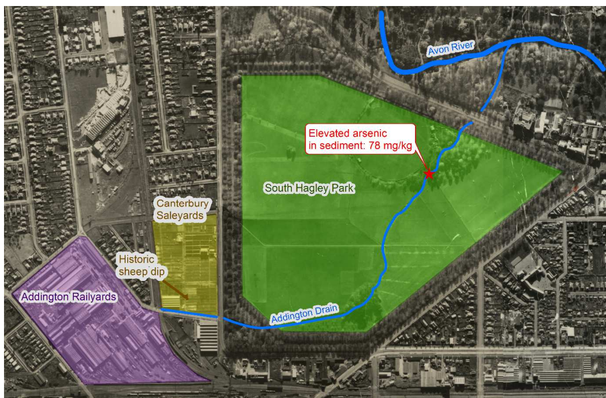
Figure 7-9: Historic landuse activities in the Addington Brook catchment that may have resulted in elevated arsenic (1946 aerial photo). Note: Aerial photo from Environment Canterbury.
