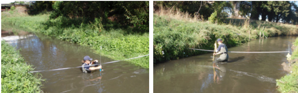
FIGURE 2 Measuring water velocity at Site 44 (left) and collecting an invertebrate sample at Site 43 (right) in the Halswell River.
