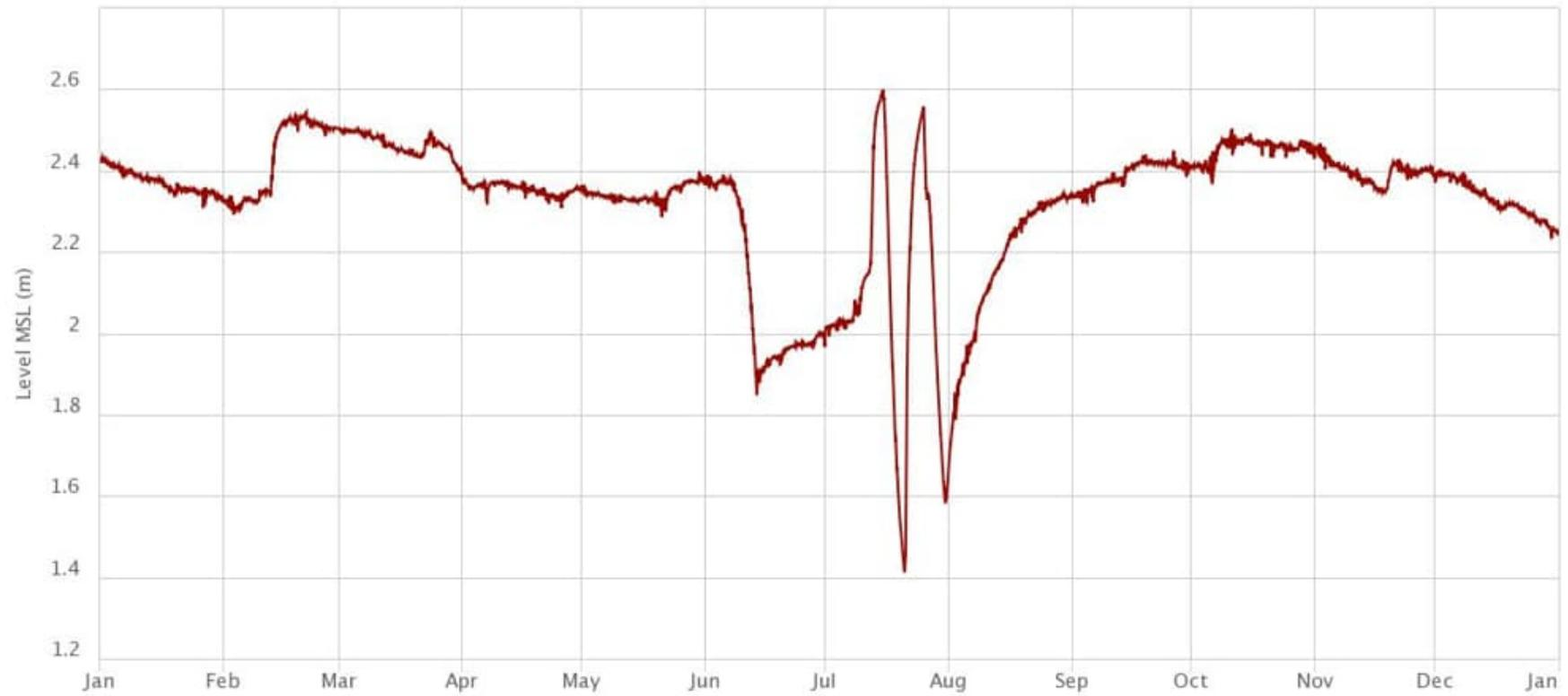
Figure 13. Water level in Te Roto o Wairewa – Lake Forsyth January – December 2022. The sharp drops in water levels indicate when the lake was opened.
