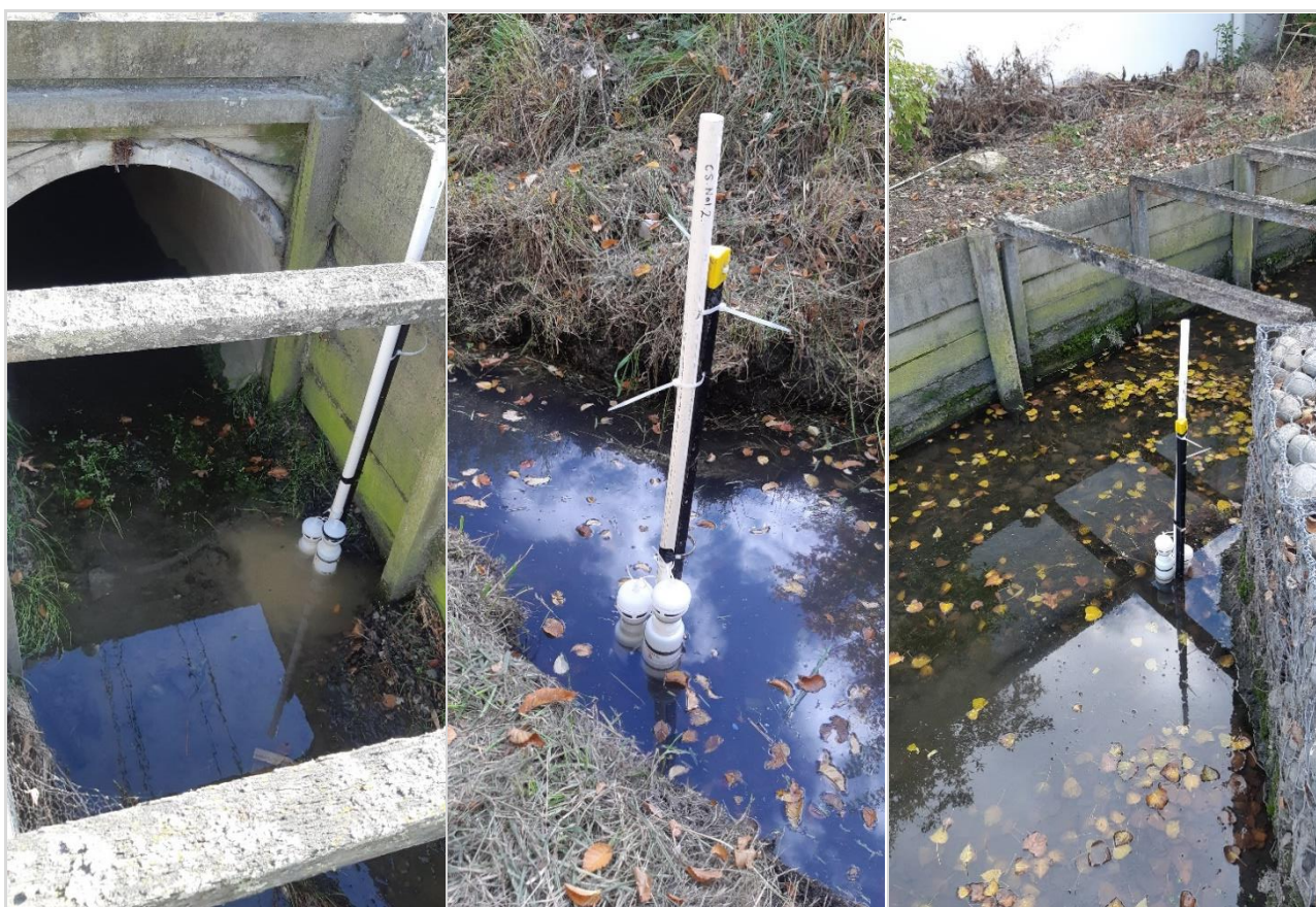
Figure 2-2: Waratah with two Nalgene sampling bottles installed at the three sampling sites. From left to right: CSNa1, CSNa2 and CSNa3.
