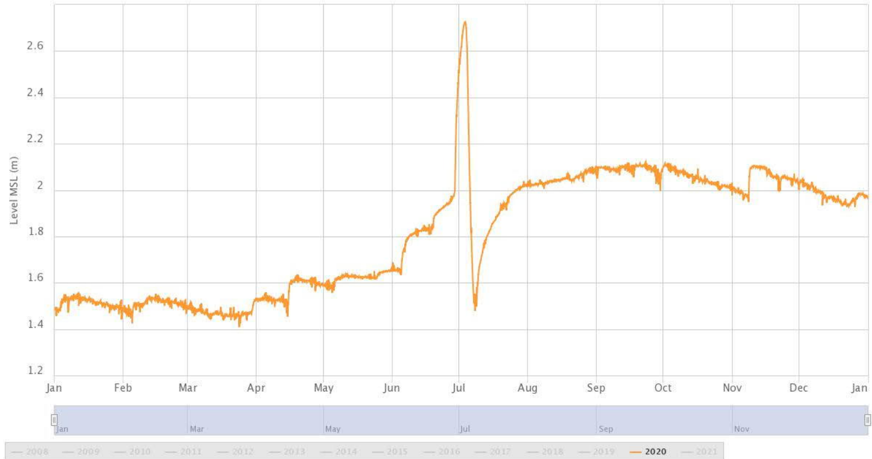
Figure 13. Water level in Lake Forsyth/Te Wairewa in 2020. The sharp drop in water level indicates when the lake was opened.
