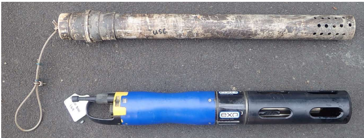
Figure 3: NEP495 (upper) and EXO3 logger (lower), both in their deployed state with protective covers on.
