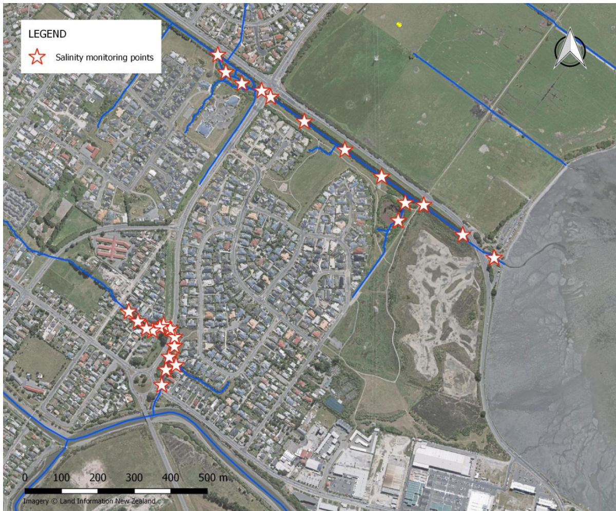
Figure 4. Location of salinity monitoring points in Linwood Canal and Steamwharf Stream.
