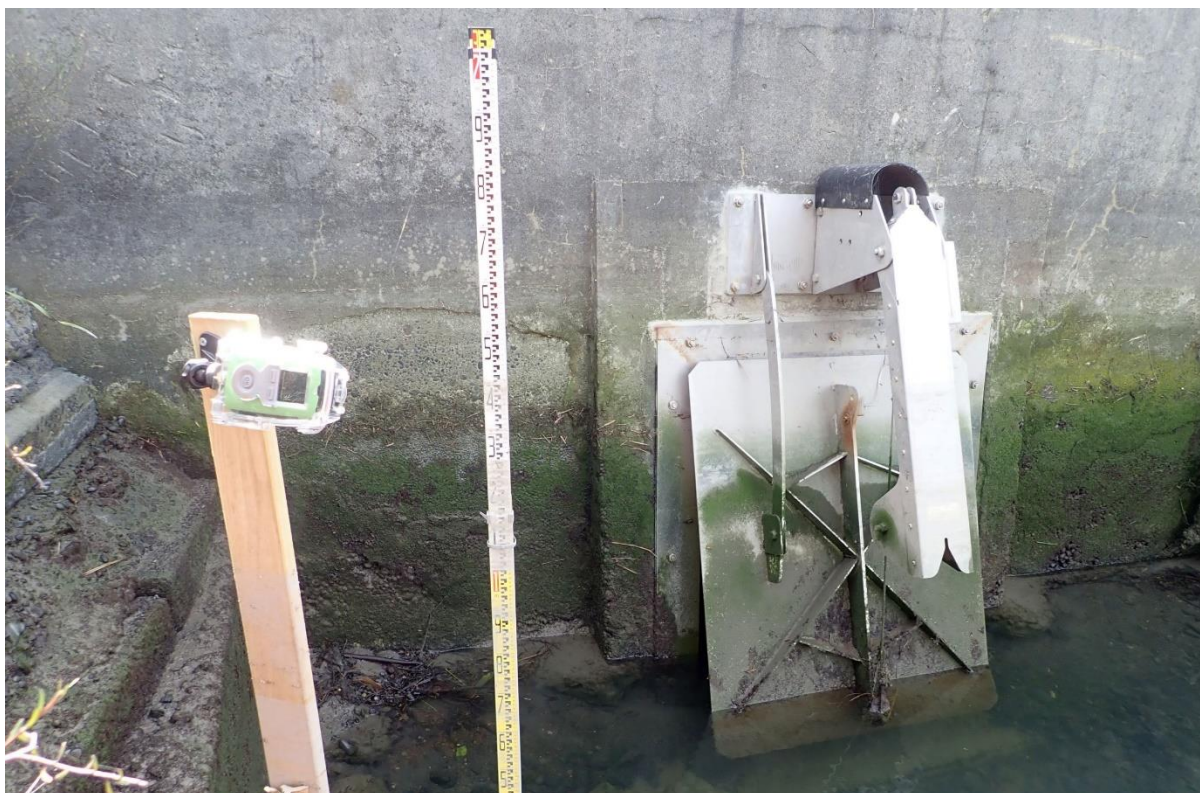
Figure 6: Time-lapse camera and temporary staff gauge setup at Steamwharf Stream.
