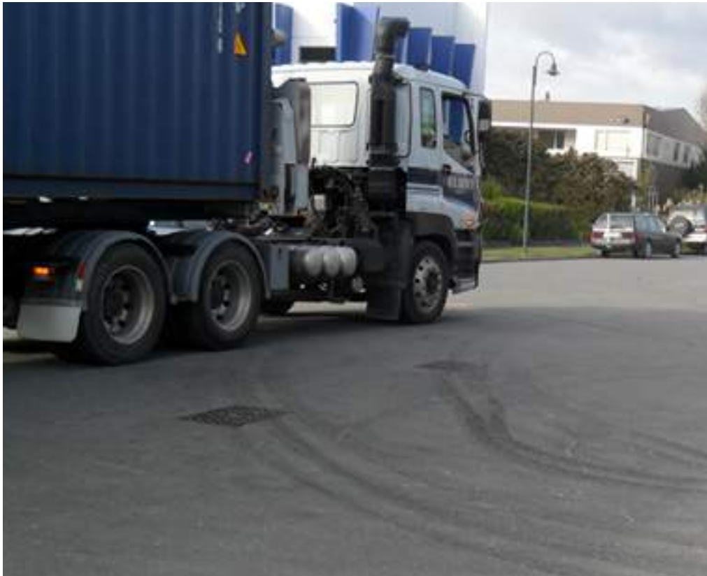
Tyre wear on the road surface is a source of contaminants
