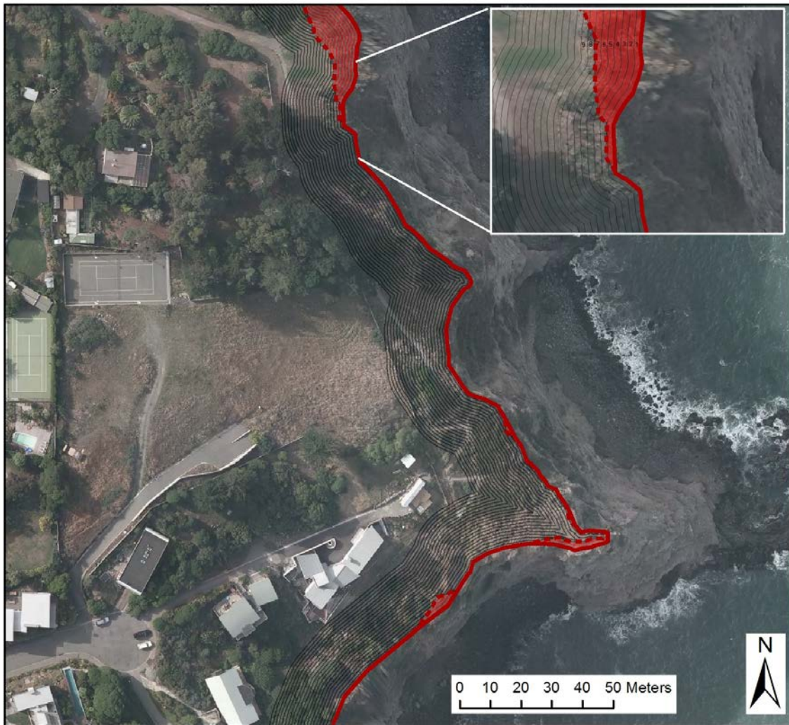
Figure 18 Example of how the area lost at the top of the cliff between the LiDAR surveys has been estimated. The solid red line represents the 2003 cliff edge and the dashed red line represents the 2011a cliff edge. The black lines with numbers (see inset) represent 1 metre zones (back from the 2003 cliff edge) that run parallel to the 2003 cliff edge. Area shown is on Whitewash Head.
