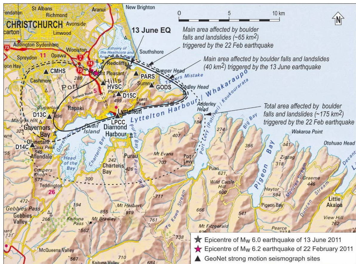
Figure 3 Location map showing the area affected by rockfalls triggered by the 2010/2011 Canterbury earthquakes (modified after Hancox et al., 2011).
