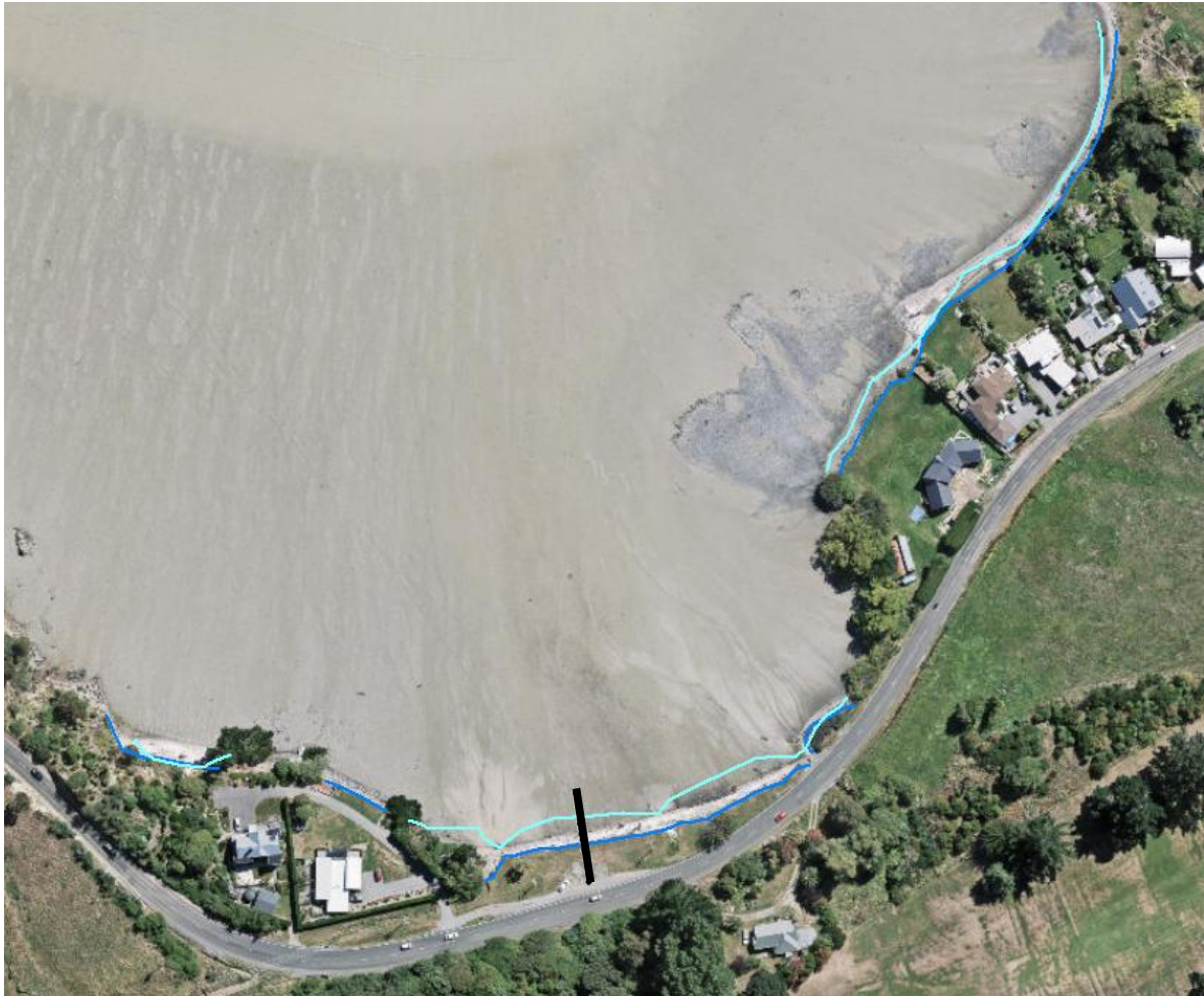
Figure G17 Southern embayment in Charteris Bay with the location of the survey transect (black line) indicated and the 1970-1974 (light blue line) and 2005-2017 shoreline (dark blue line) derived from aerial imagery (source: Canterburymaps.govt.nz )
