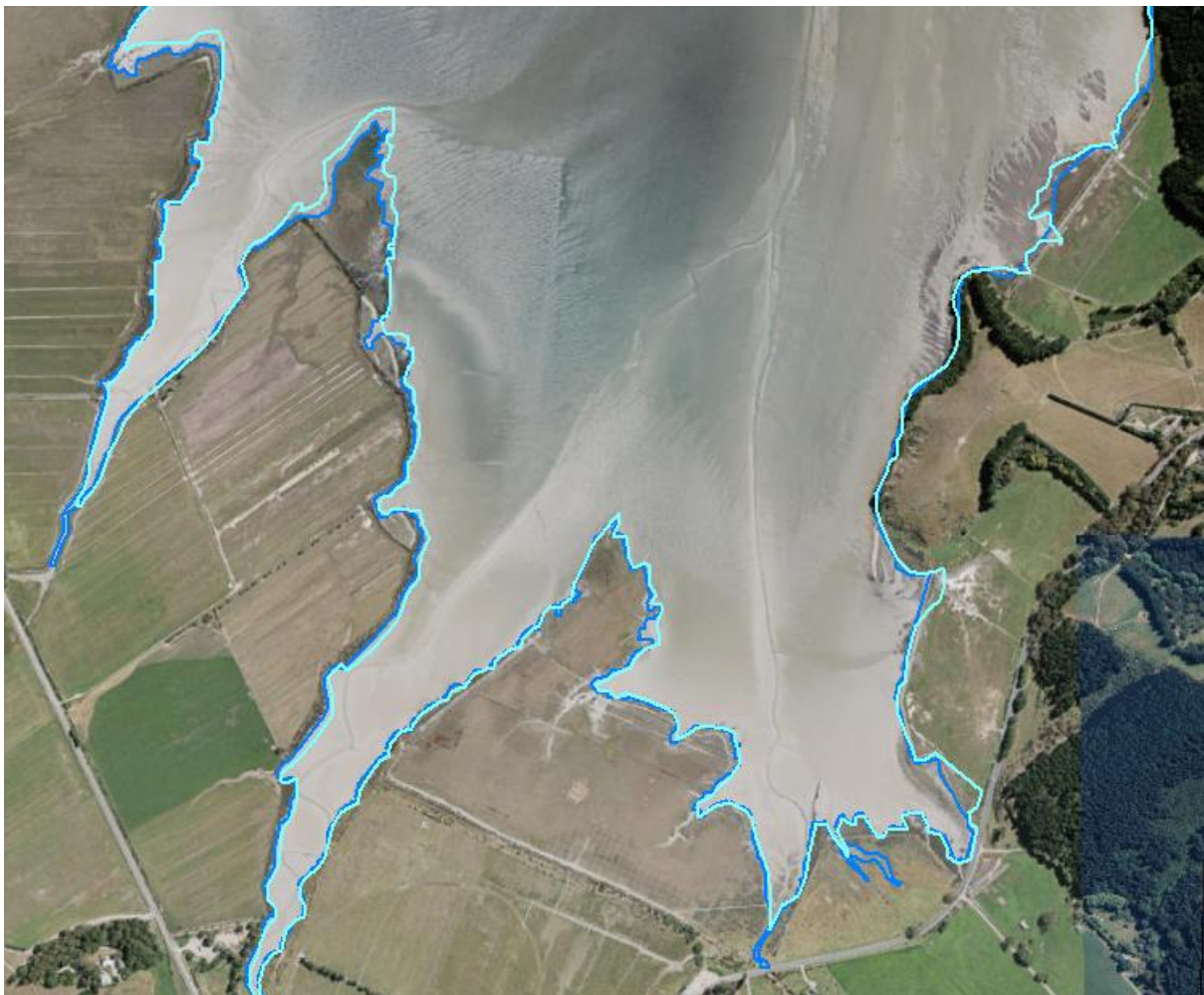
Figure G14 Satellite image of the Teddington shoreline with the 1970-1974 (light blue line) and 2005-2017 shoreline (dark blue line) derived from aerial imagery (source: Canterburymaps.govt.nz )
