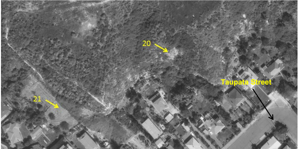
Figure 8 1984 aerial photograph, showing gullies A and B and several areas of bare ground/possible landslide scars (numbered).
