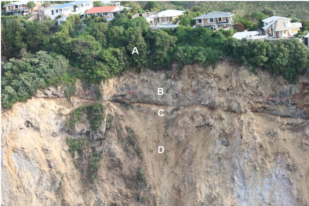
Figure 9 View to the west onto the northern cliff at Wakefield Avenue. The homes are accessed from Richmond Hill Road. The loess/fill, which is thickly covered by tall shrubs, overlies rock at the slope crest ( A ). The rock exposed in the upper part of the cliff ( B ) is columnar jointed basalt lava and breccia. The persistently recessed layer beneath this is the epiclastic deposit ( C ), and the material below this is massive trachy basalt lava breccia ( D ). Photograph C. Massey GNS Science (July 2011).
