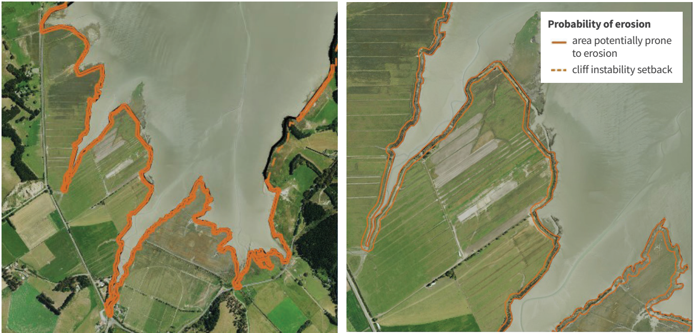
Coastal storm erosion distances with 40cm of sea level rise – sourced from Coastal Hazard Assessment 2021 (Tonkin & Taylor). The orange areas show the areas potentially prone to coastal erosion.
