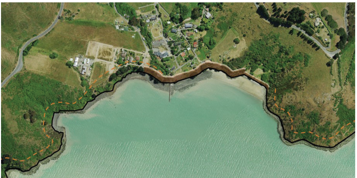
This image shows the probability of storm term erosion with 40cm of sea level rise. The dashed orange lines represent areas of cliff prone to future instability. The brown areas are where more detailed assessment has been undertaken and show the probability of short-term storm erosion – sourced from Coastal Hazard Assessment 2021 (Tonkin & Taylor).
