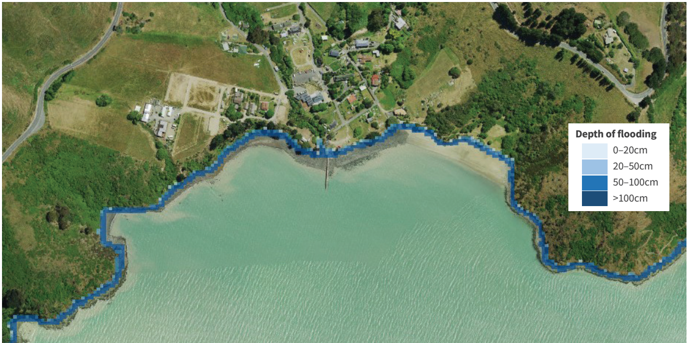
Coastal flooding extent and depths with 40cm of sea level rise during a rare (1 in 100 year) storm event – sourced from Coastal Hazard Assessment 2021 (Tonkin & Taylor).
