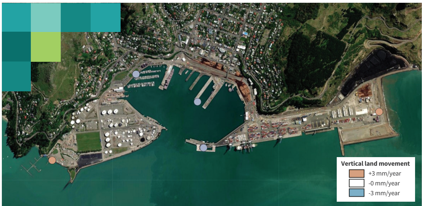
Some areas are shown to be subsiding and others to be uplifting (Source: NZ SeaRise). There is uncertainty associated with this data, so this information should be considered indicative only.
