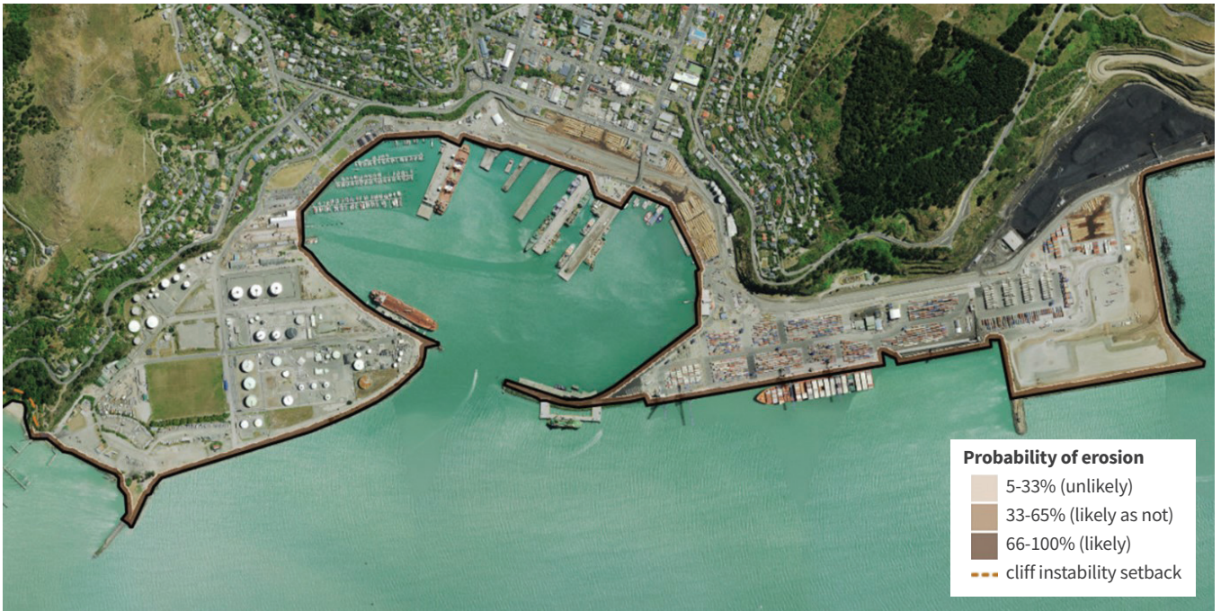
This image shows the probability of storm erosion occurring with 40cm of sea level rise, sourced from Coastal Hazard Assessment 2021 (Tonkin & Taylor). The brown areas show the probability of short-term storm erosion. The dashed orange line shows the area of bank/cliff prone to future instability.
