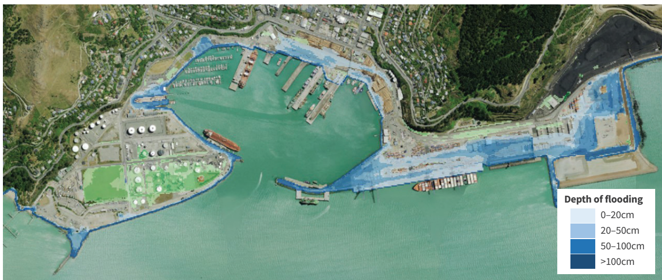
Coastal flooding extent and depths with 40cm (top) and 1m (bottom) of sea level rise during a rare (1 in 100 year) storm event – sourced from Coastal Hazard Assessment 2021 (Tonkin & Taylor). Indirect flooding is shown in green.
