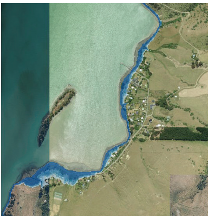
Coastal flooding extent and depths with 40cm (left) and 1m (right) of sea level rise during a rare (1 in 100 year) storm event - sourced from Coastal Hazard Assessment 2021 (Tonkin & Taylor).
