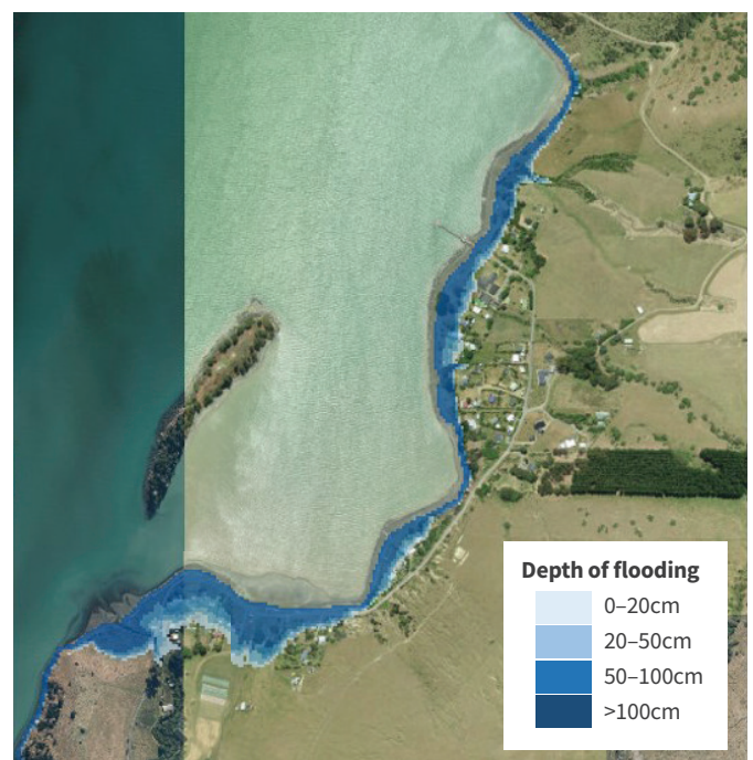
Coastal flooding extent and depths with 40cm (left) and 1m (right) of sea level rise during a rare (1 in 100 year) storm event - sourced from Coastal Hazard Assessment 2021 (Tonkin & Taylor).
