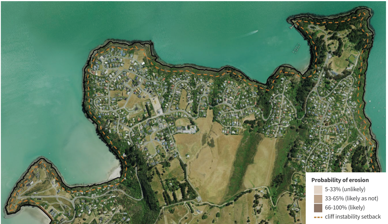
The dashed orange lines represent areas of cliff prone to future instability – sourced from Coastal Hazard Assessment 2021 (Tonkin & Taylor).
