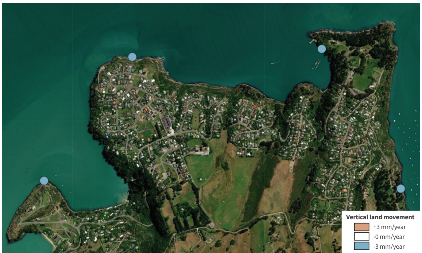
Land is shown to be subsiding, as per blue-coloured dots (Source: NZ SeaRise). There is uncertainty associated with this data, so this information should be considered indicative only.
