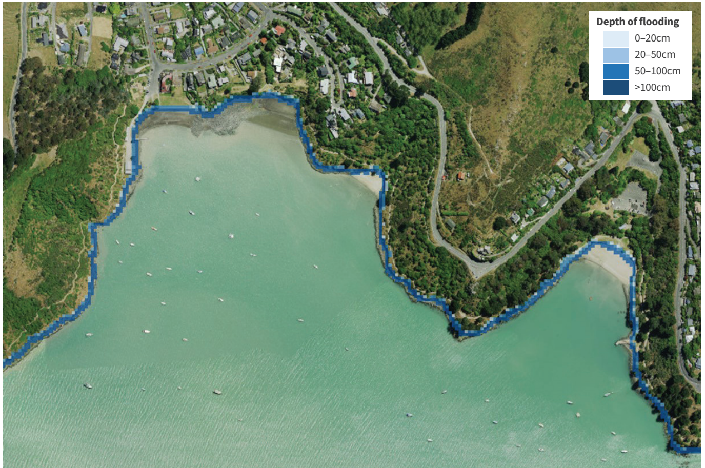
Coastal flooding extent and depths with 40cm of sea level rise during a rare (1 in 100 year) storm event – sourced from Coastal Hazard Assessment 2021 (Tonkin & Taylor).
