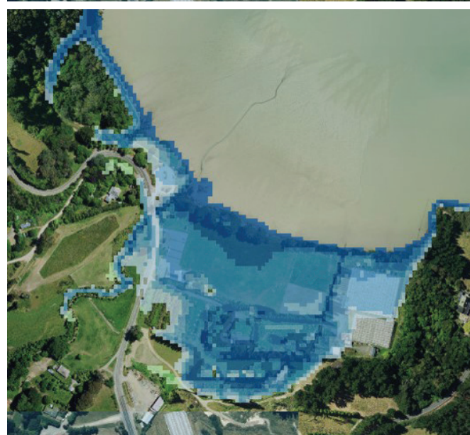
Coastal flooding extent and depths with 40cm (top) and 1m (bottom) of sea level rise during a rare (1 in 100 year) storm event – sourced from Coastal Hazard Assessment 2021 (Tonkin & Taylor). Indirect flooding is shown in green.
