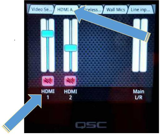
Note: To MUTE sound touch either button located under volume slides Once you have finished, remove the cable from the wall and laptop QSC Touchpad will shut down automatically
