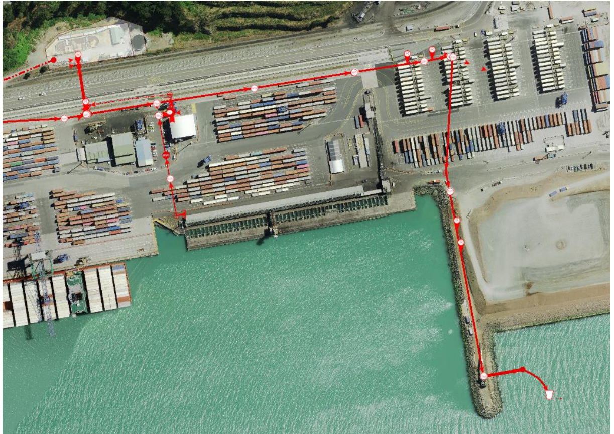
Figure 1: Location of CCC's wastewater pipelines within LPC's land holding and showing containers and hardstand. Image from CCC's GIS ( https://gis.ccc.govt.nz/portal/apps/webappviewer/index.html?id=c4ff85ba75724391ae89fbf5f773e00d ) on 14/01/2022.
