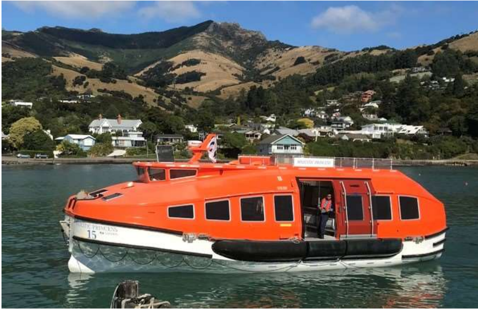
Photograph 3 – An example of a cruise ship tender (15.7m LOA, 5.2m beam)
