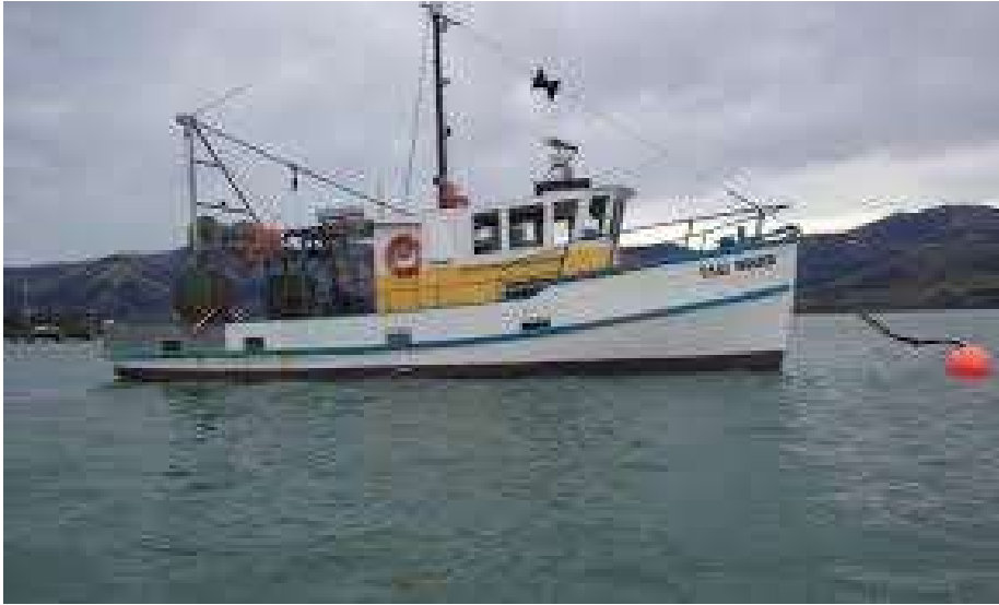
Photograph 1 – An example of a commercial fishing vessel (12m LOA, 4m beam)
