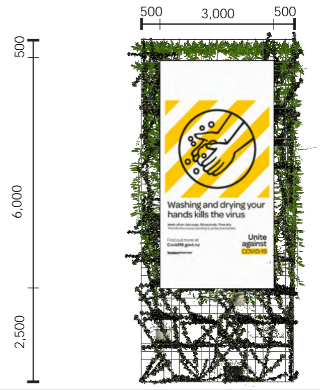
C. ELEVATIONS FOR 4m x 6m DIGITAL BILLBOARD Scale 1:100 @ A3
