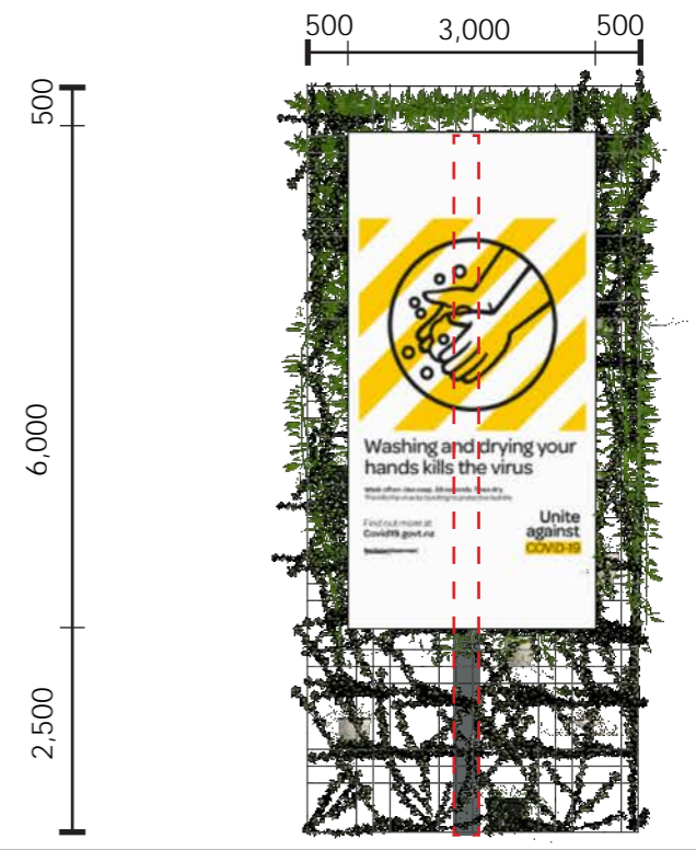
C. ELEVATIONS FOR 3m x 6m DIGITAL BILLBOARD Scale 1:100 @ A3
