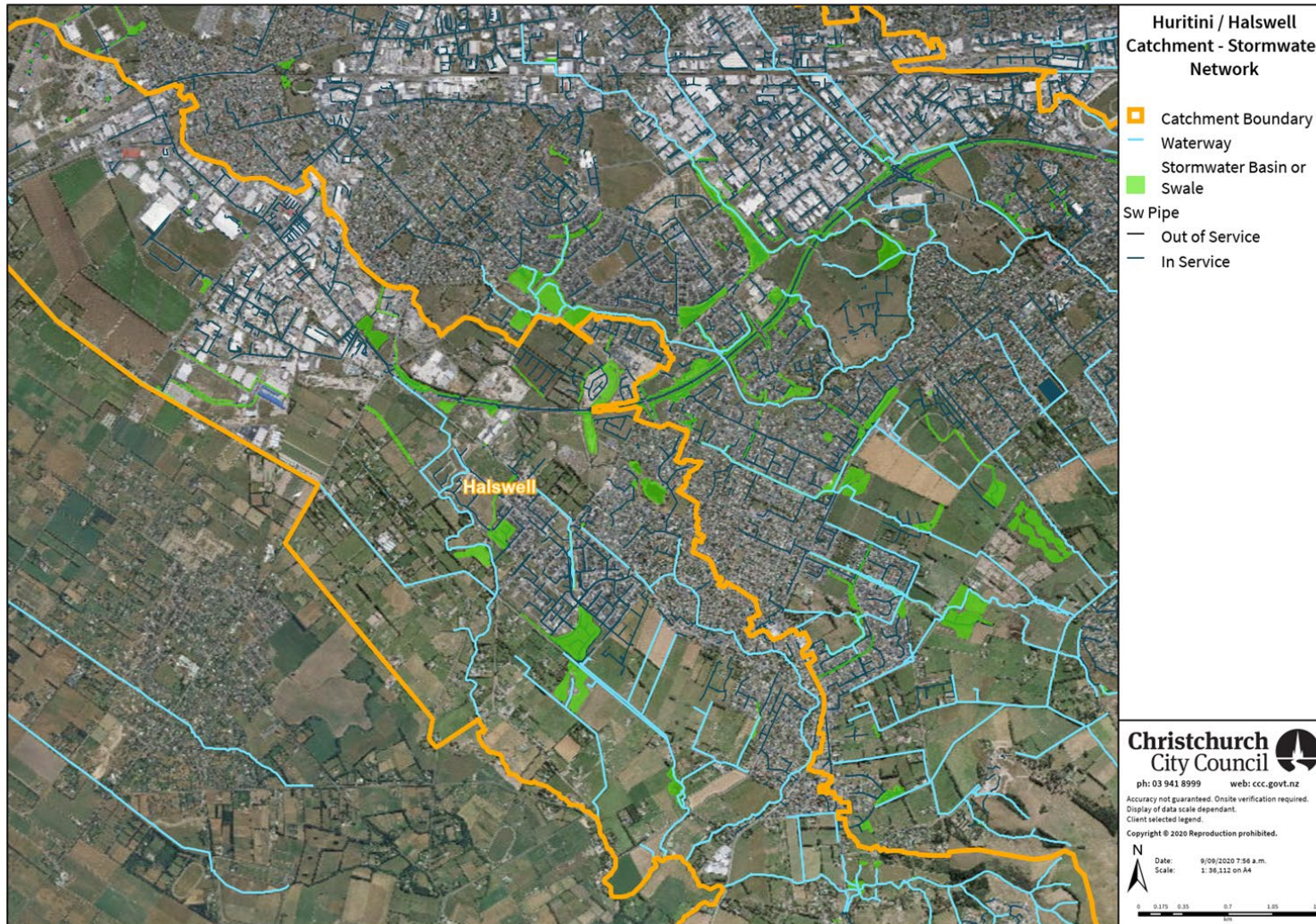
FIGURE 5: STORMWATER NETWORK MAP
