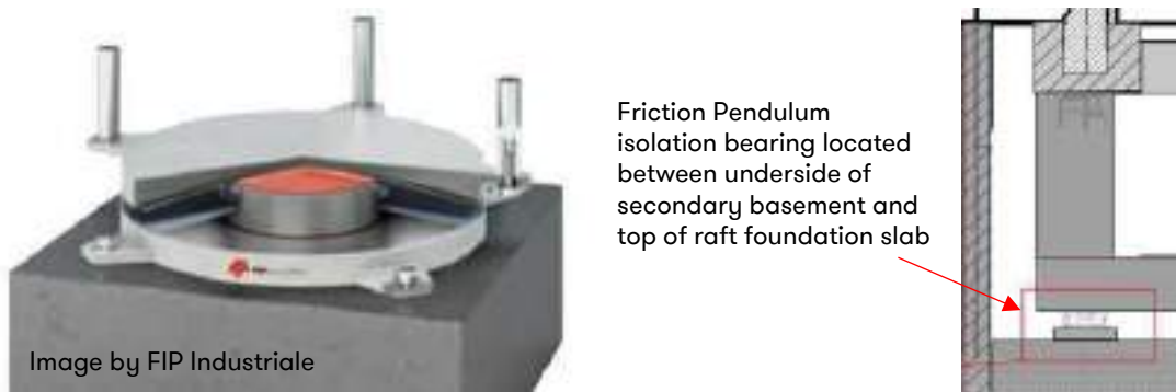
Figure 1. (a) Example of a friction pendulum isolation bearing (b) schematic basement section indicating location of isolator and approximate structural element build-up.
