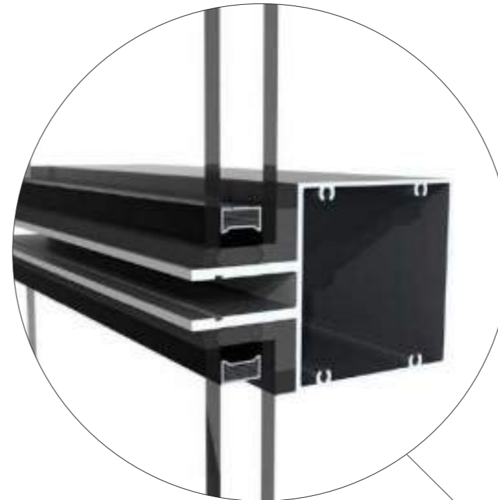
APL Structural Glaze Suite transom & mullion 3D details, box section 125mm or 168mm depending on structural loading design
