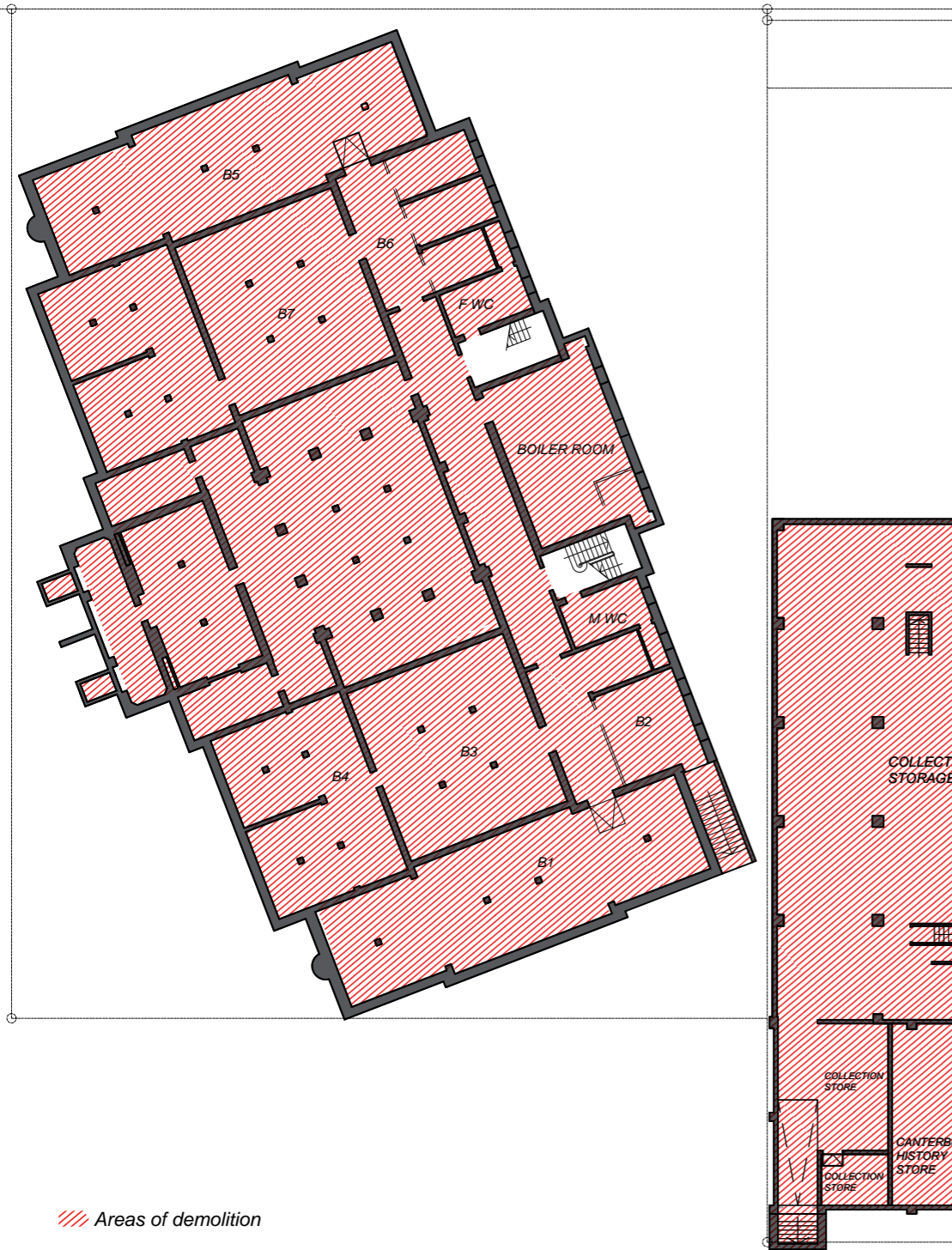
Demolition floor plan
