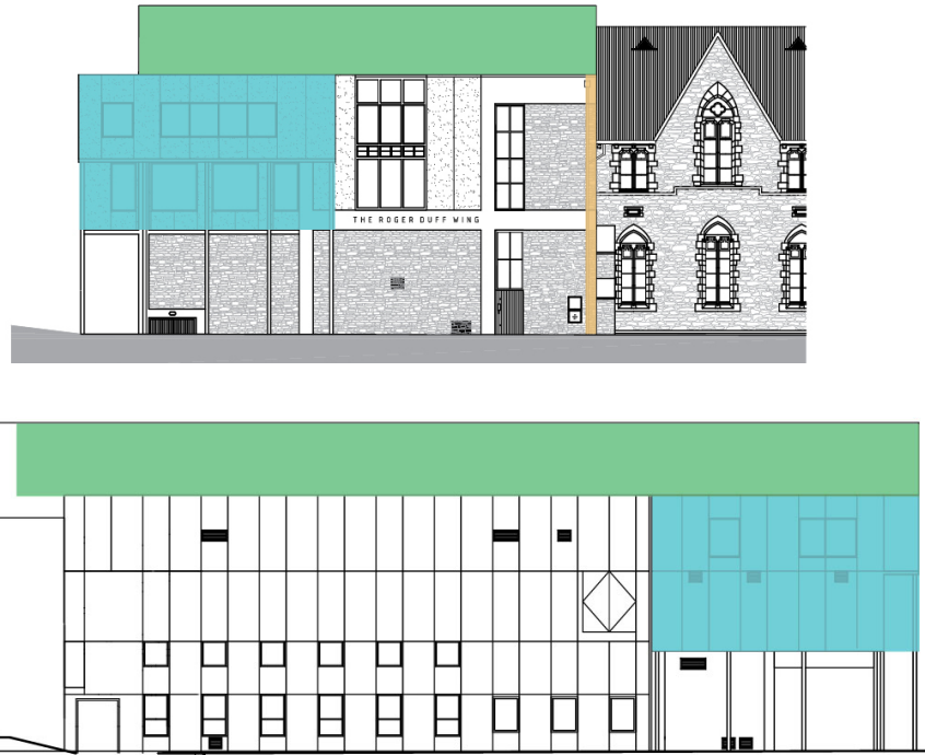
Image 29: Current 1977 facades, with highlighted areas requiring design considerations with the redevelopment. It should be noted that the reason there are numerous design consideration to this public face of the Museum is that the majority of the other public faces are the more highly significant Mountfort buildings.
