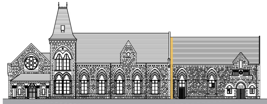
Image 11: Existing Rolleston Avenue Museum Plan & Elevation. Area in orange indicates the extent of 1958 façade & roof fabric removal for the separation in context with the whole Rolleston Avenue façade.
