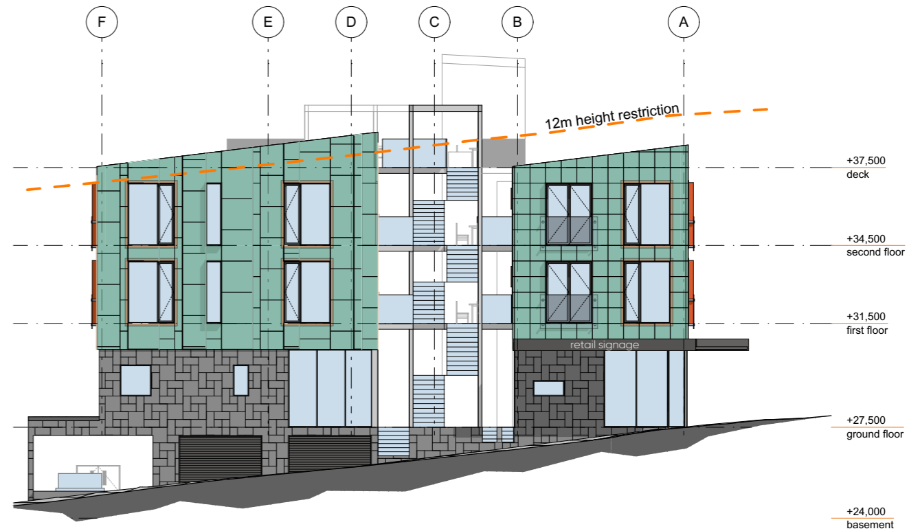
04 east elevation scale 1:200 @ A3
